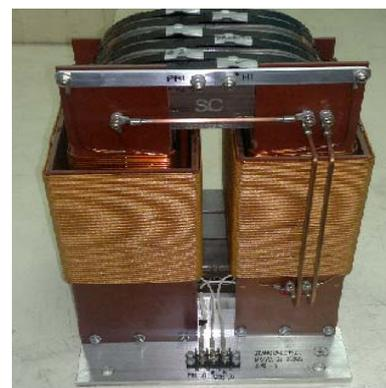
Fig. 5: Pulse Transformer with 1:4 turns ratio
