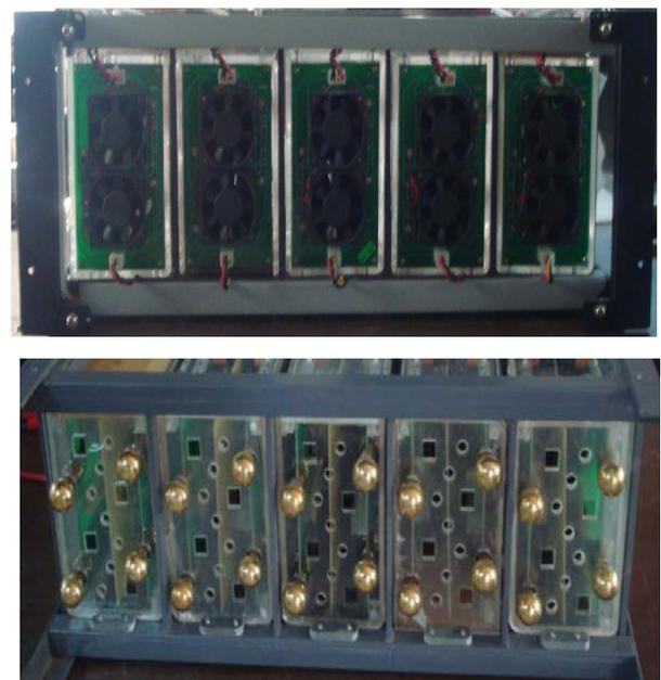
Fig. 2: Solid state modulator front and back view
